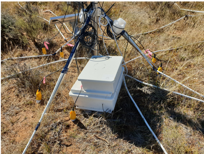
Figures (left above and below). New experimental setup of oxygen sensors at the Middelburg field site ( right above and below ) Eddy Covariance flux tower at the Middelburg field site. Photos: Justin du Toit
