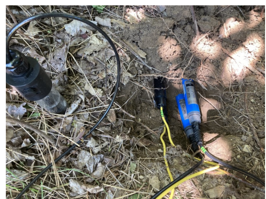
Figures (above left) Overview of the overall setup and the arrangements of sensors at each of the three stations, (below left) Setting up the power supply and the logger, (above right) An apple tree in the fruit orchard equipped with a sap flow sensor, (below right) One of the six measurements points. Two types of TDRs are installed next to each other and adjacent to TDR profile sensors (plastic tube). The matric potential sensors are on the other side of the tube.
