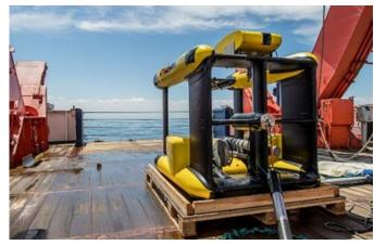
*Figure 2 (above).* The TRIAXUS, a towed remotely controlled underwater vehicle.
