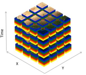
**Figure**. The Open Date Cube project is an open source geospatial data management and analysis software project supported by numerous organizations including the USGS and CEOS. It is a framework for creating data cubes. Here a conceptual representation indicates a multi-dimensional stack in space, time and type of spatially aligned pixels.
